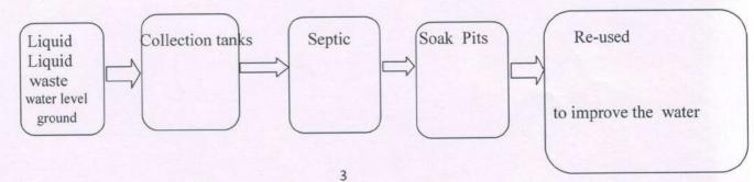
Soak pits are constructed nearby each and every septic tank for collecting the liquid waste from septic tanks and is used for soaking the water in ground and the remaining waste solid material that collects on the surface of the soak pits is dumped to deep earth pits for preparing the bio fertilizers for usage in the gardens of the campus periodically.
